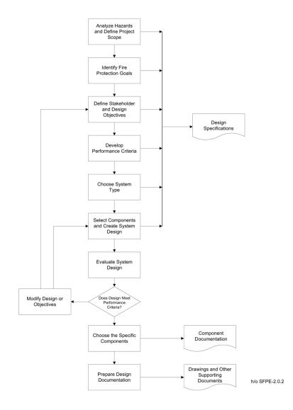
The fire alarm system designer who follows this concept applies a methodical procedure. Not only does this procedure help ensure that the results meet the specific needs of the project, but it also provides a comprehensive solution to whatever fire protection problems the procedure has identified.
