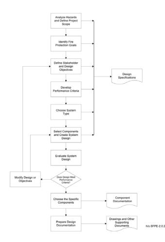
As I have suggested previously, a fire alarm system designer who intends to work in the performance-based building design arena will do well to understand that "a process makes it work." The methodical procedure makes certain that a designer will include every detail necessary to create *and* thoroughly document a design.
